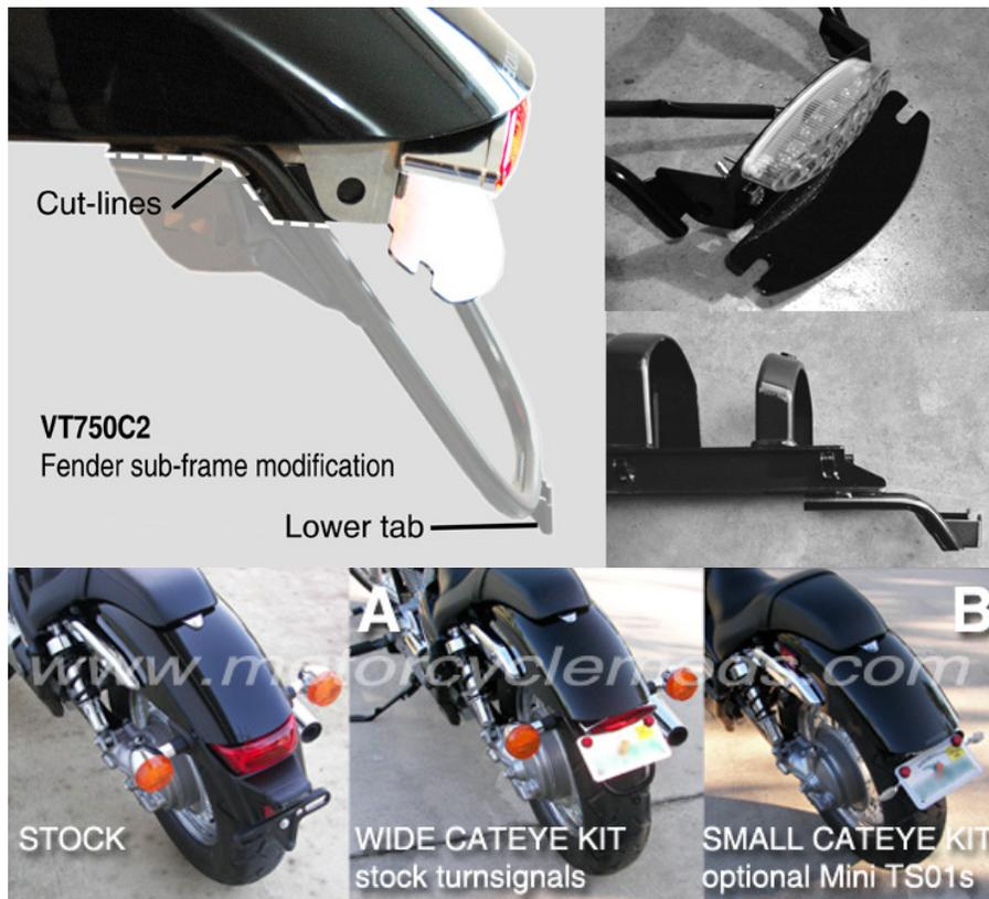
Figure A. shows the Wide Cateye Taillight, with stock turnsignals.
